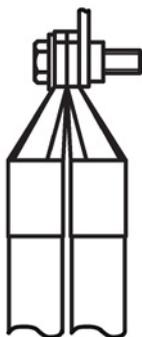
Figure 4-2 2 cable lugs per connection
