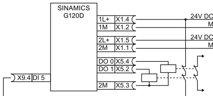
Figure 3-15 Connecting a relay at the F-DO
