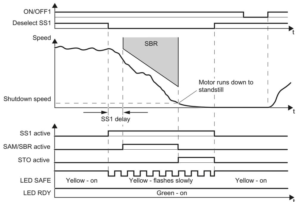
Figure 5-2 Braking behavior and diagnostics of the safety function SS1 (Safe Stop 1)
