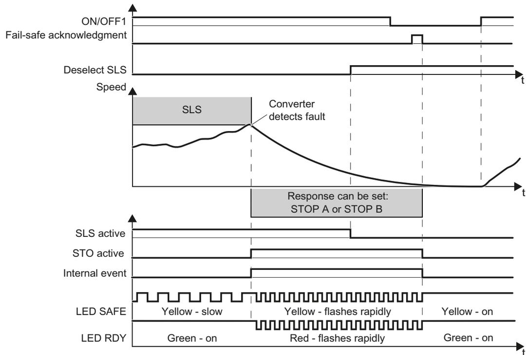
Figure 5-45 Fault response of the SLS safety function
