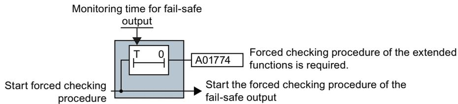
Figure 4-14 Start and monitoring of the forced checking procedure of the fail-safe output
