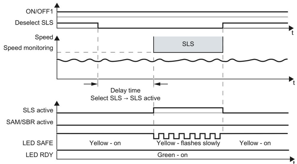
Figure 5-7 Selecting and deselecting the SLS safety function at low speeds
