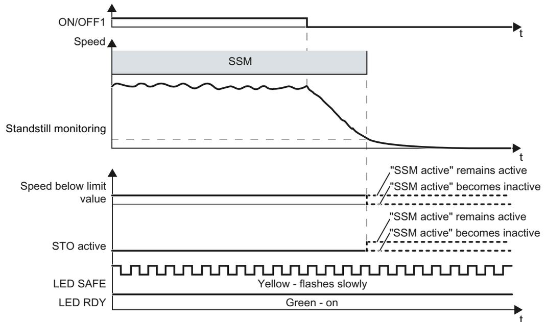
Figure 5-16 OFF1 command when the SSM safety function is active
