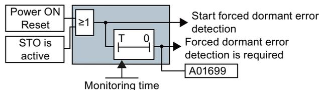
Figure 4-4 Triggering and monitoring the forced checking procedure
