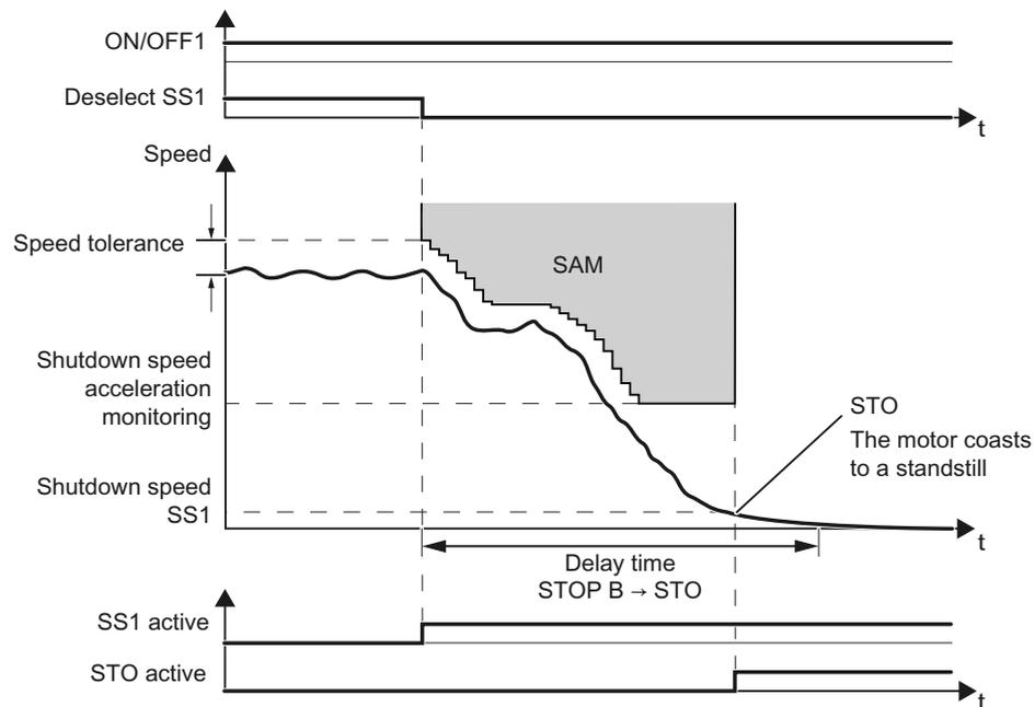
Figure 4-16 SS1 with acceleration monitoring
