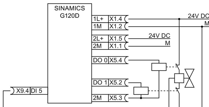
Figure 3-16 Connecting the F-DO of the G120D, mode3
