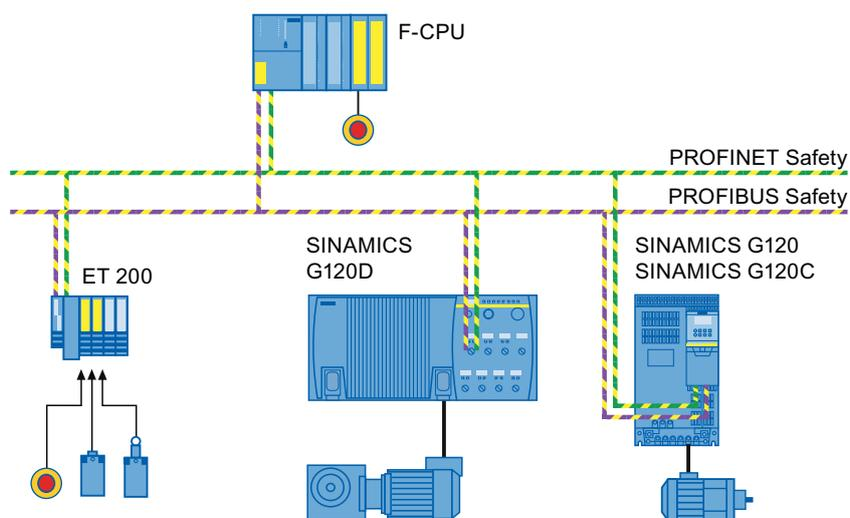
Figure 3-18 PROFIsafe communication between F-CPU and converter
