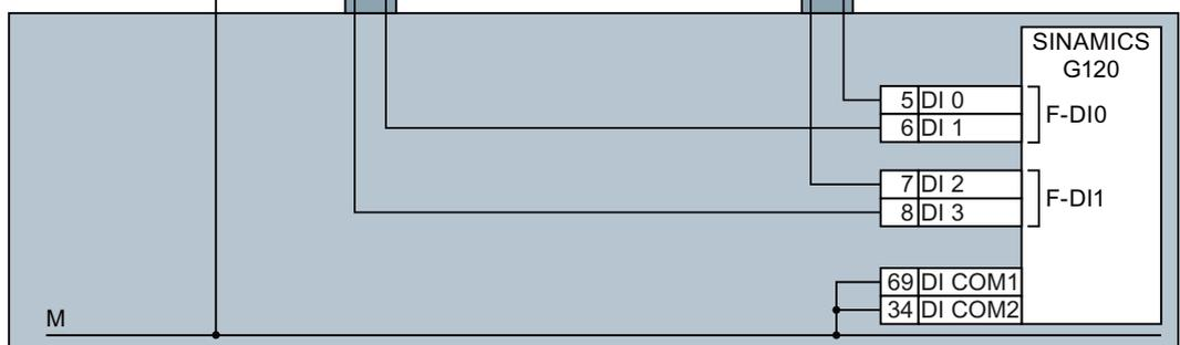
Figure 3-10 Interconnecting the converter and Modular Safety System in separate control cabinets
