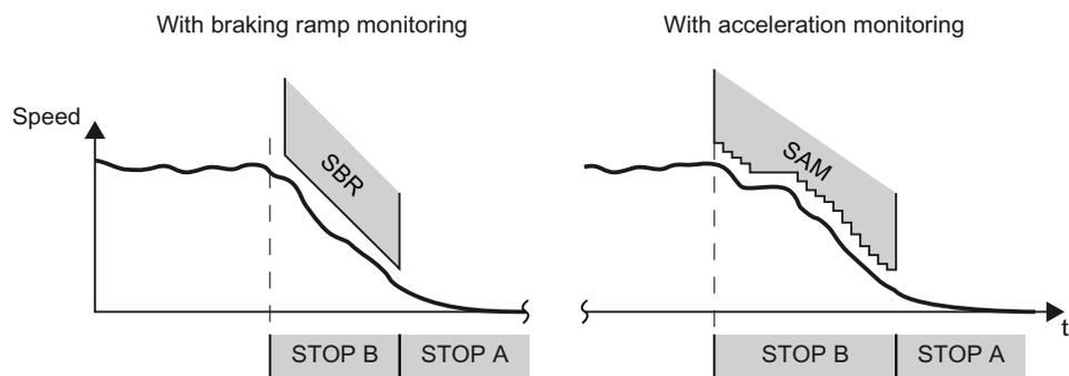
Figure 5-36 Monitoring the speed for a STOP B
