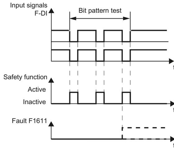
Figure 4-2 Converter response to a bit pattern test
