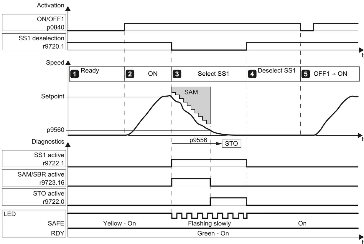
Figure 4-28 SS1 acceptance test with acceleration monitoring
