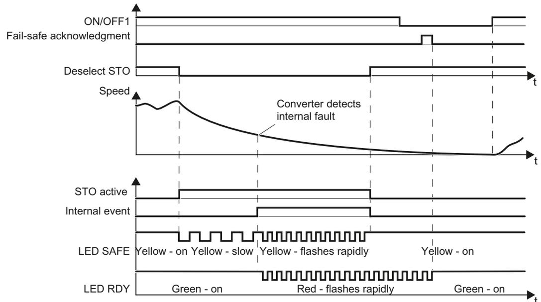
Figure 5-42 Internal event when the STO safety is active
