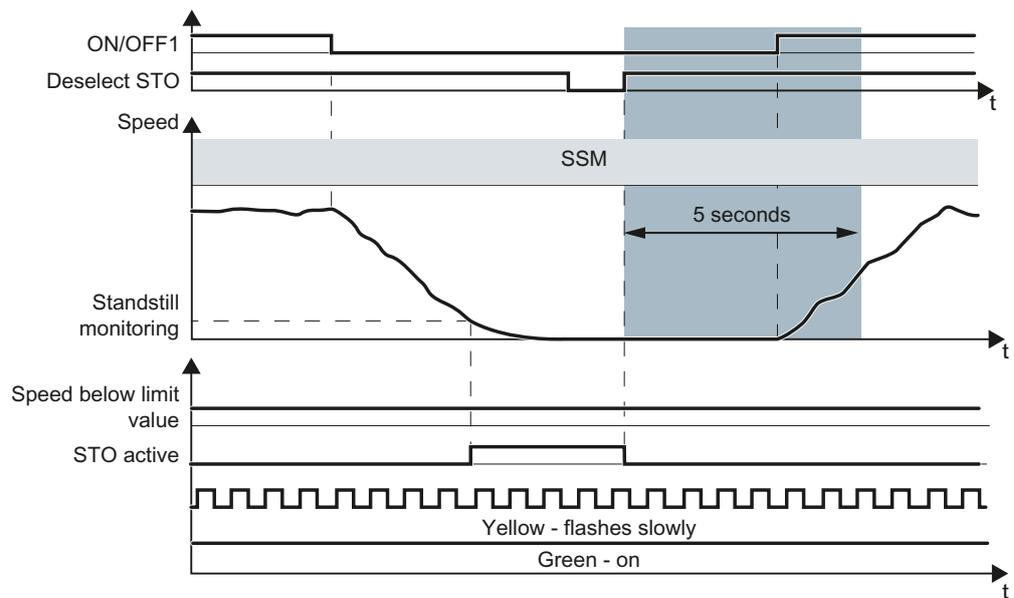
Figure 5-20 Switching the motor off and on with SSM active
