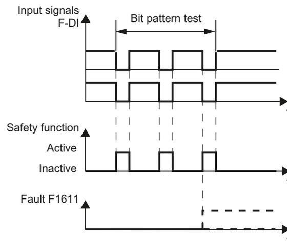
Figure 4-9 Converter response to a bit pattern test
