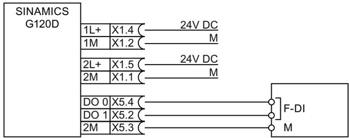
Figure 3-17 Connecting the F-DO of the G120D, mode4
