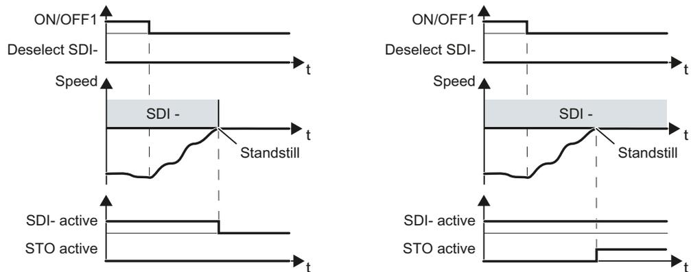
Figure 4-22 Behavior when the motor is switched off. Left: SDI becomes inactive. Right: SDI remains active
