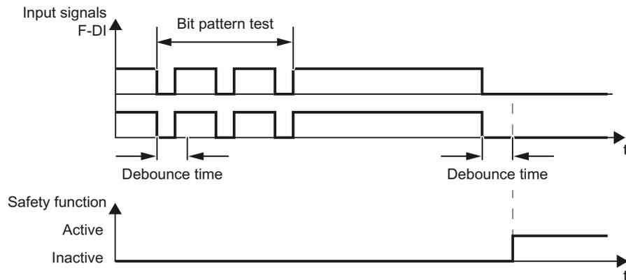
Figure 4-3 Filter for suppressing temporary signal changes
