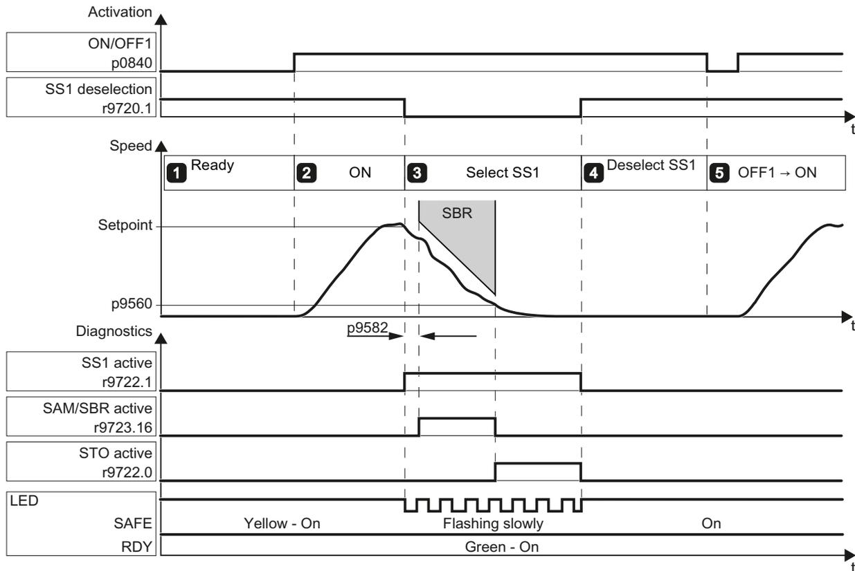
Figure 4-27 SS1 acceptance test with braking ramp monitoring
