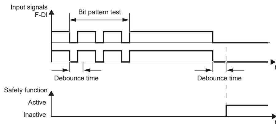
Figure 4-10 Filter for suppressing temporary signal changes
