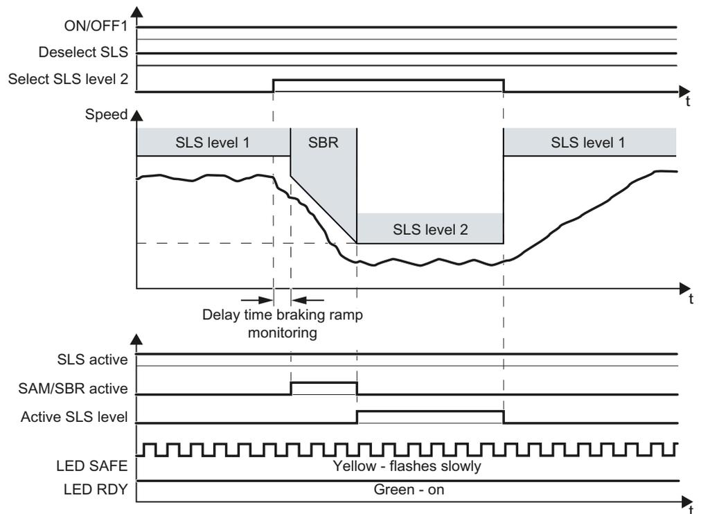
Figure 5-6 Switching between different monitoring thresholds
