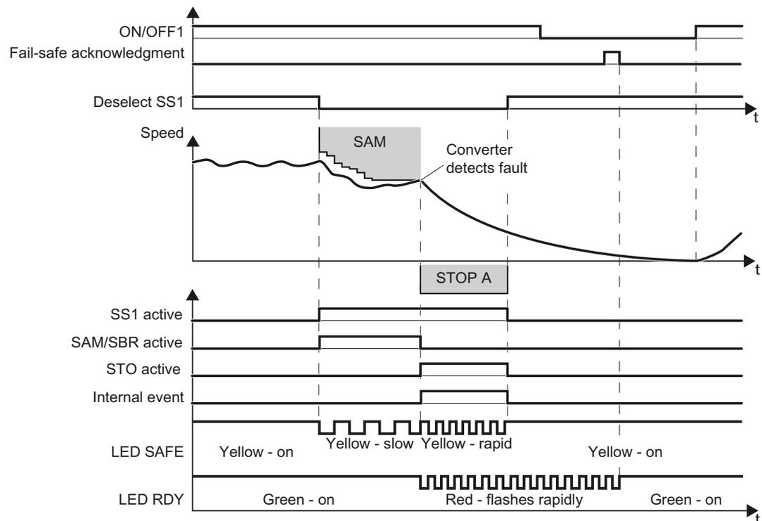
Figure 5-44 General fault response of safety function SS1 (as example: SS1 with acceleration monitoring)
