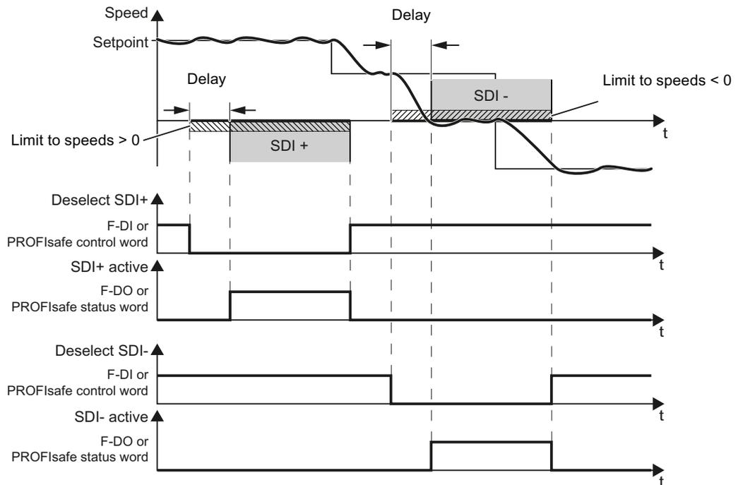
Figure 2-2 Time response of the safety function SDI (Safe Direction)
