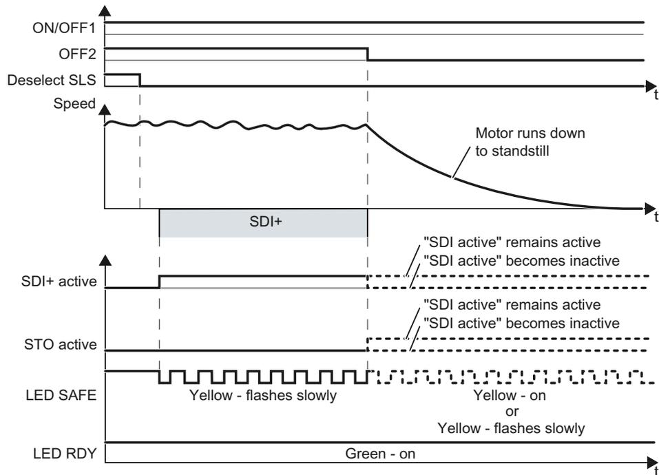
Figure 5-22 OFF2 command while the SDI safety function is active
