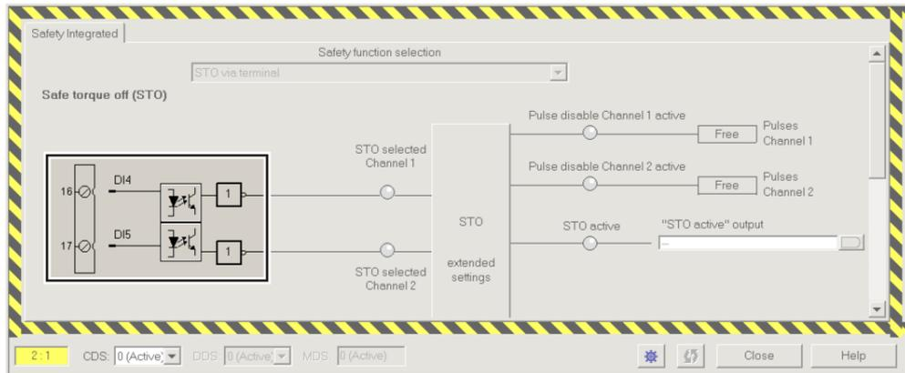
Figure 4-5 Example: automatic assignment of digital inputs DI 4 and DI 5 with STO
