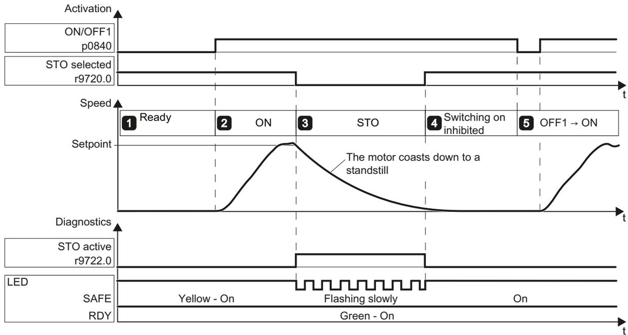
Figure 4-26 STO acceptance test for extended functions
