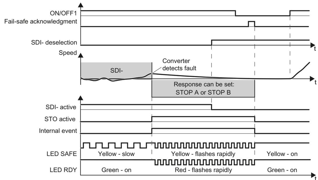
Figure 5-46 Fault response of the SDI safety function
