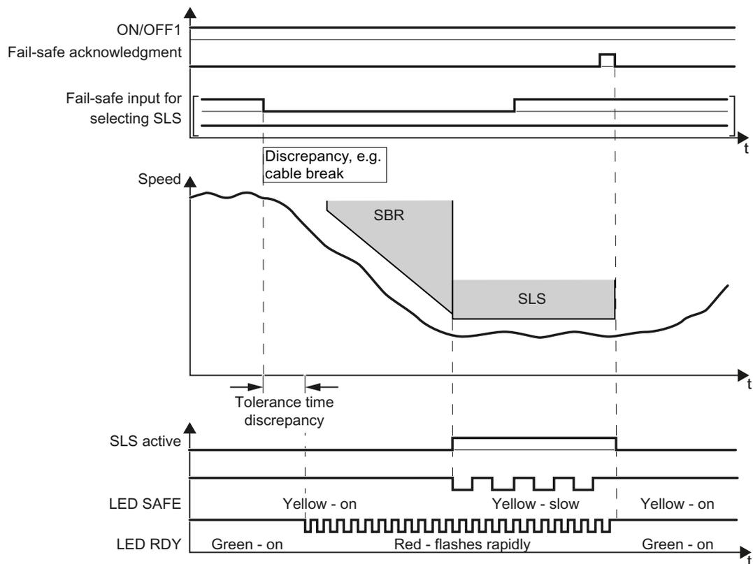
Figure 5-40 Response of safety function SLS in the event of a discrepancy
