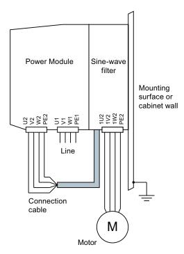
Figure 7-6 Connecting the sine-wave filter as base component
