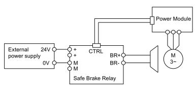
Figure 7-9 Safe Brake Relay connection
