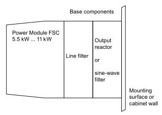
Figure 7-1 Mounting base components
