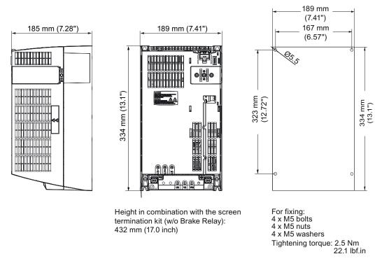
Figure 3-2 Dimensions and drill pattern, FSC (HO 5.5 kW ... 11 kW)
