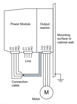
Figure 7-4 Connecting the output reactor as base component
