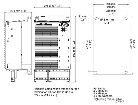
Figure 3-5 Dimensions and drill pattern, FSE unfiltered (HO 30 kW ... 37 kW)
