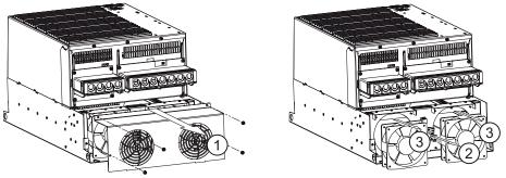
Figure 5-3 Cooling fan removal FSF (45 kW ... 75 kW)
