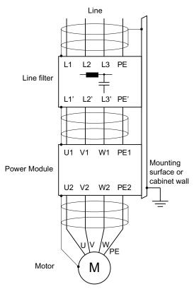
Figure 7-3 Connecting the line filter as lateral component
