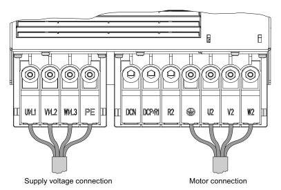
Figure 4-4 Power and motor terminals FSD ... FSF
