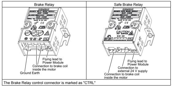
Connect the other end of the cable form to the Power Module
