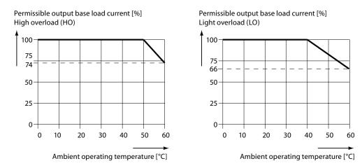
Figure 6-1 Current derating for temperature
