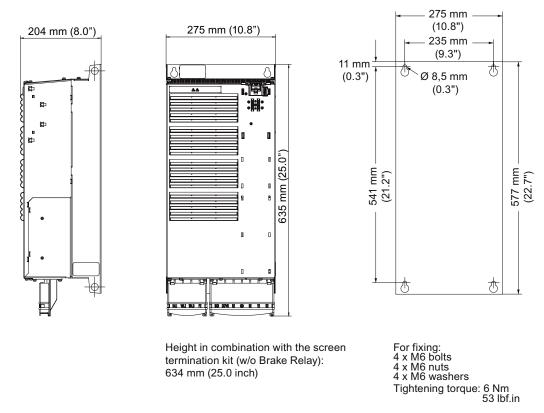
Figure 3-6 Dimensions and drill pattern, FSE filtered (HO 30 kW ... 37 kW)
