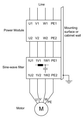
Figure 7-7 Connecting the sine-wave filter as lateral component
