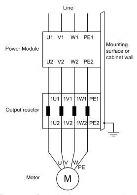
Figure 7-5 Connecting the output reactor as lateral component
