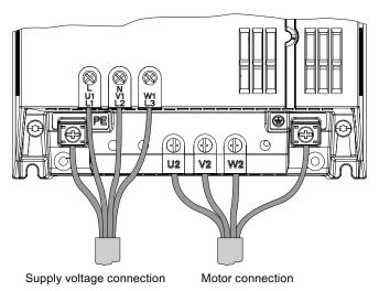
Figure 4-3 Power and motor terminals FSC
