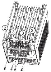
Figure 5-1 Cooling fan removal FSC (5.5 kW ... 15 kW)
