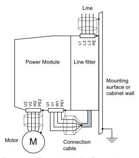
Figure 7-2 Connecting the line filter as base component
