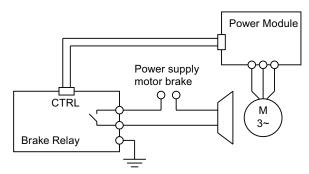
Figure 7-8 Brake Relay connection
