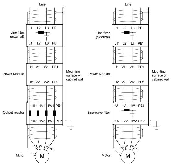
Connecting power components with output reactor
