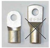
Ensure that the terminals cover can be closed, if two cables are connected to the same terminal. An inverter with open terminals cover provides only IP00 protection level.
