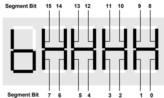
The significance of the relevant bits in the display is described in the status and control word parameters.
