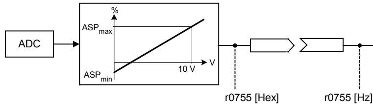
$$r0755 [\text{Hz}] = \frac{r0755 [\text{Hex}]}{4000 [\text{Hex}]} \cdot P2000 \cdot \frac{\max(|\text{ASP}_{\text{max}}|, |\text{ASP}_{\text{min}}|)}{100\%}$$
