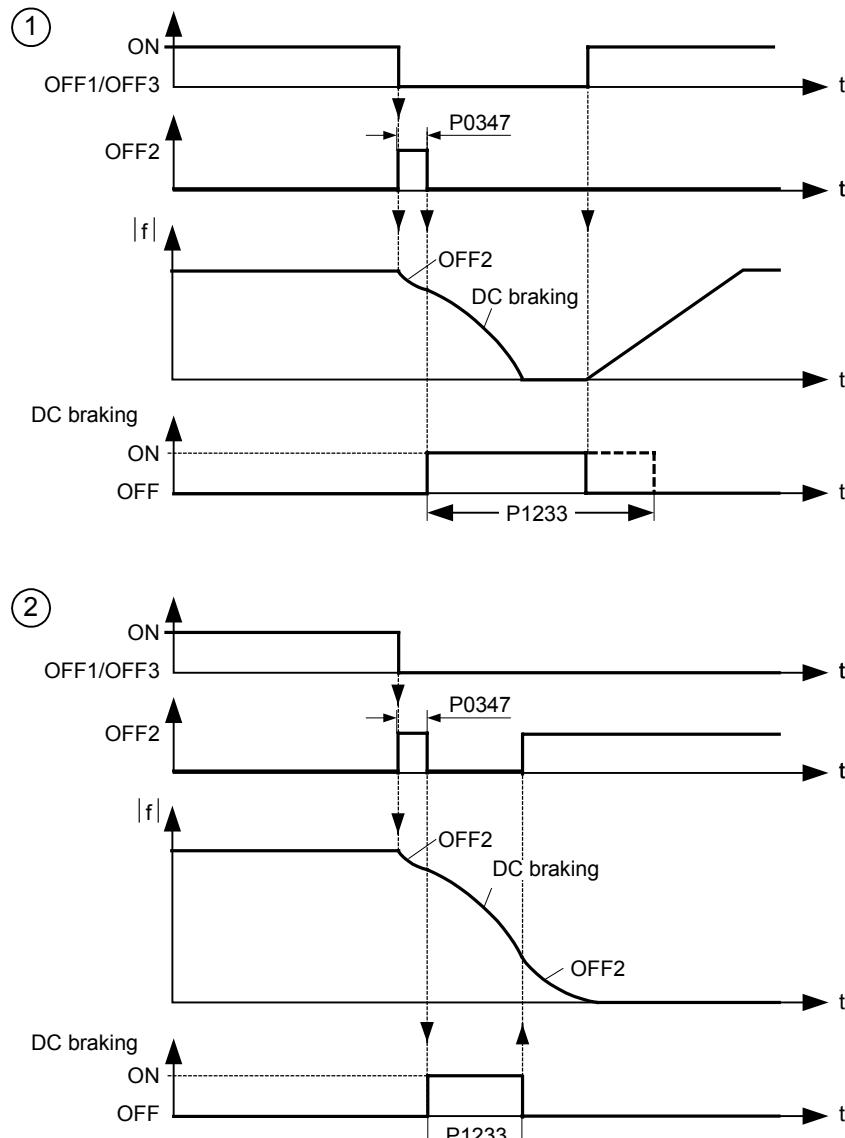
Parameter P1233 still controls the level of DC injection.
