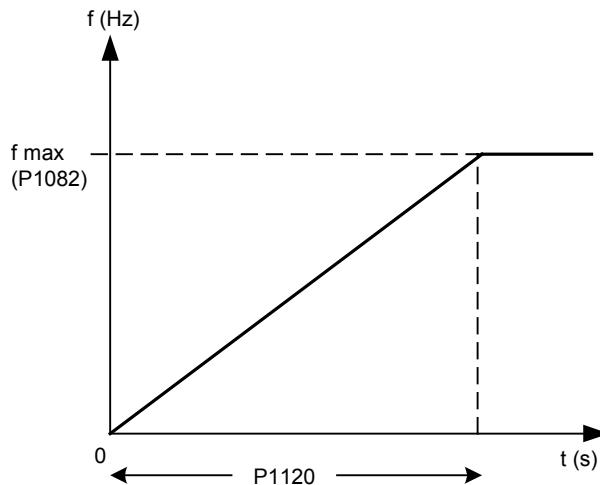
Setting the ramp-up time too short can cause the inverter to trip (overcurrent).
