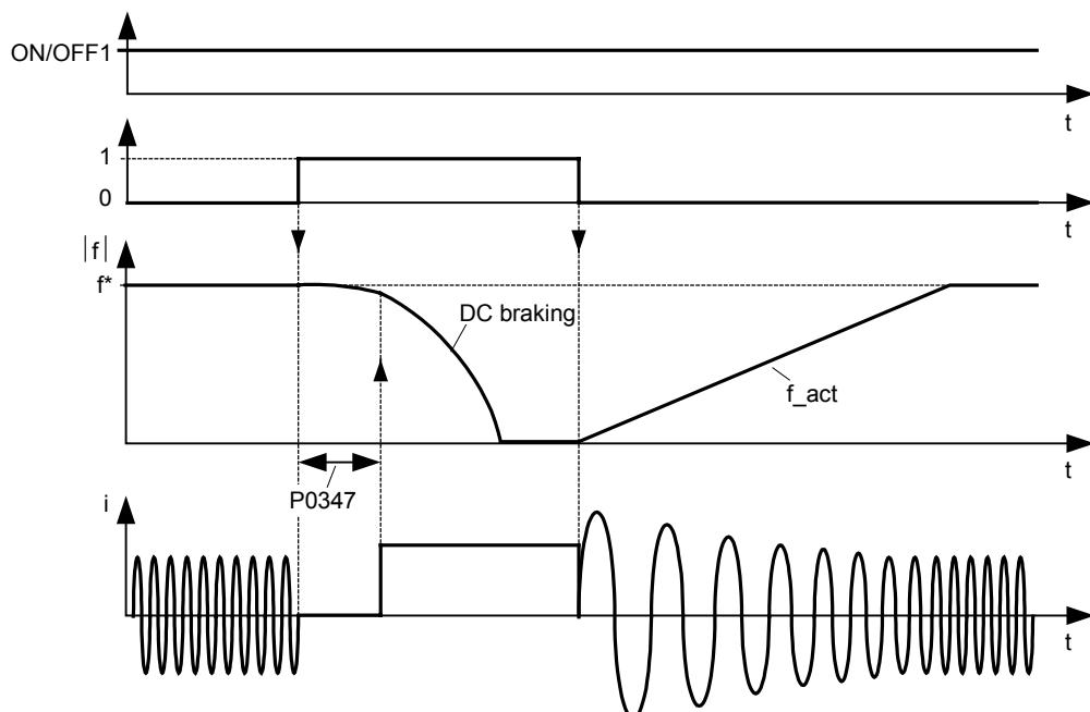
The level of DC braking is set in P1232 (DC braking current - relative to the rated motor current) which is set to 100 % by default.
