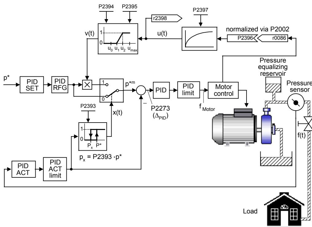
If the active current falls below the normalized threshold  $P2395$ , then the setpoint is linearly decreased as a function of the active current.
