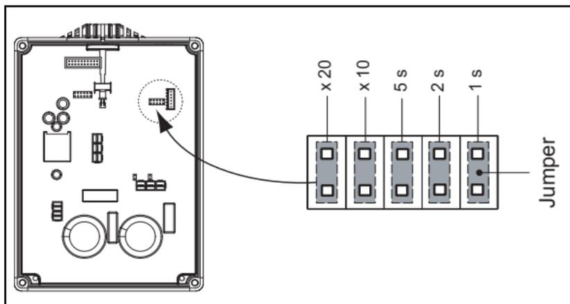
Figure 8 Ramp Times Using Jumpers
