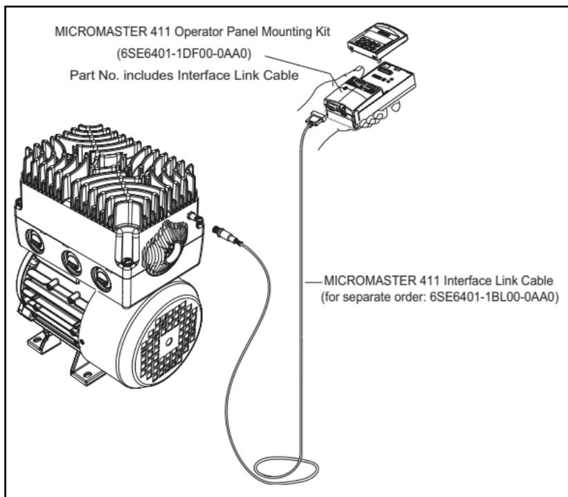
Figure 10 BOP / AOP connected to MICROMASTER 411
