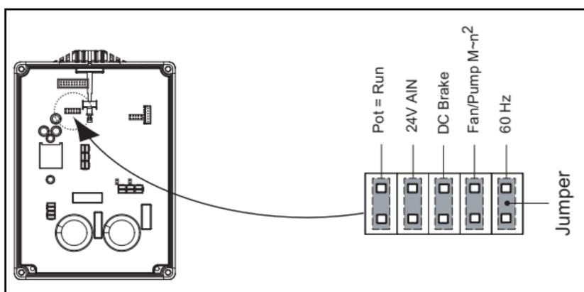
Figure 9 Control Circuit Jumpers
