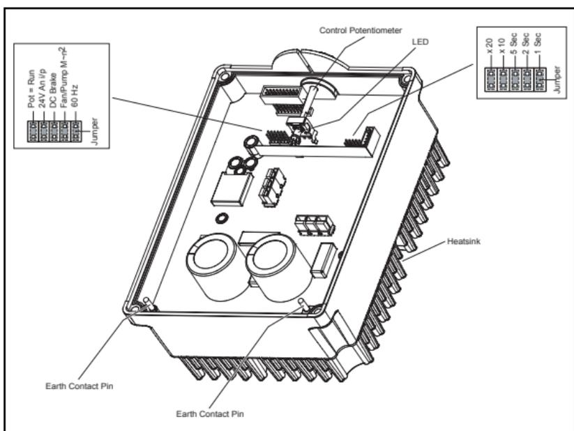
Figure 2 MICROMASTER 411 Inverter Cover (Case Size B)
