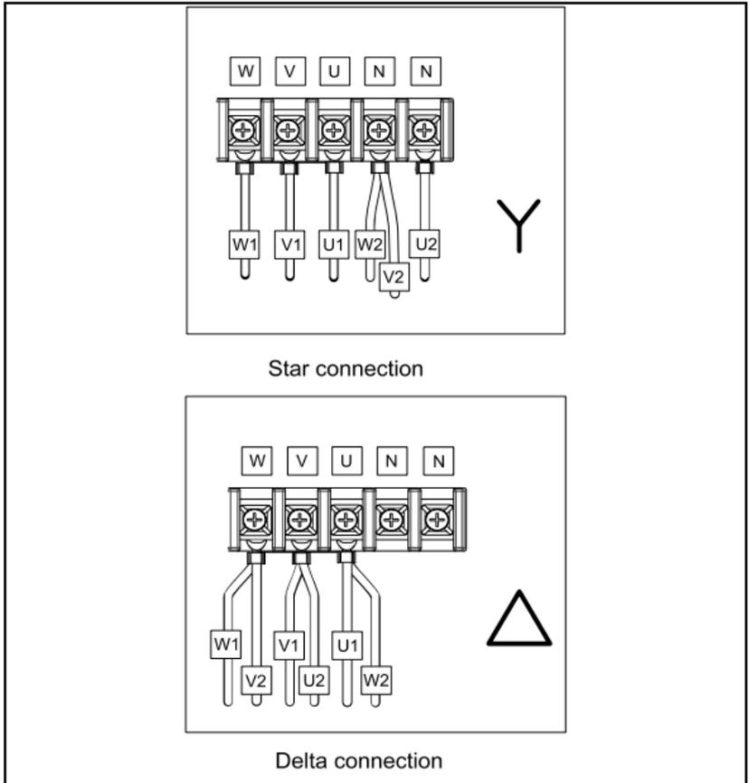
Figure 5 Star / Delta Connections
