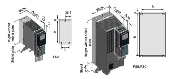
Table 3-1 Dimensions depend on the Control Unit (CU) and HMI device [mm]
