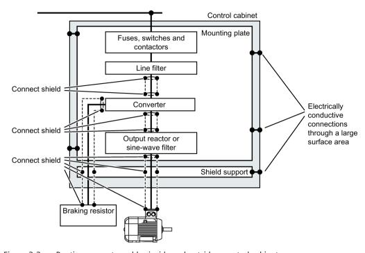
Figure 3-3 Routing converter cables inside and outside a control cabinet
