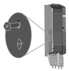
Figure 4-2 Remove screw for functional grounding
