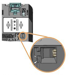
Brake relay connector for FSA ... FSC Power Modules without STO terminals
