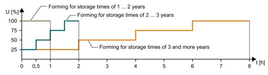
Figure 5-2 Forming the DC-link capacitors
