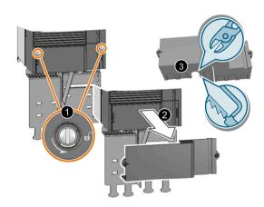
FSF, FSG: Remove the lower cover
