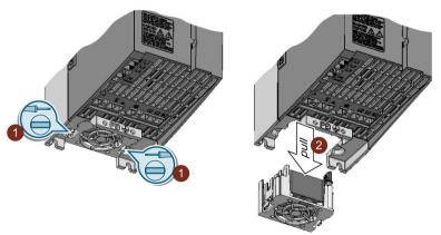
4. Install the new fan module in the inverse sequence.
