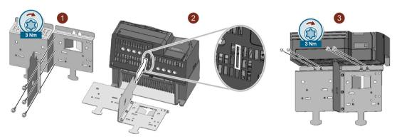
You have correctly mounted the EMC connecting bracket and the shield plate.
