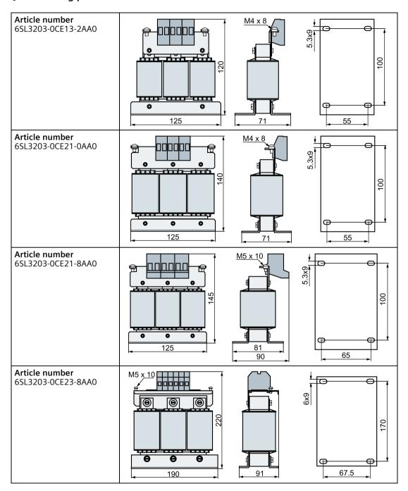
Mount the line reactor using M5 screws, nuts and washers. Tightening torque: 6 Nm
