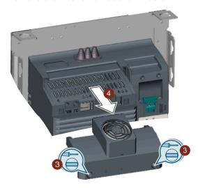
3. Install the new fan module in inverse sequence.
