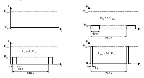
Figure 8-6 Pulse power, rated power and examples of the switch-on duration of the braking resistor
