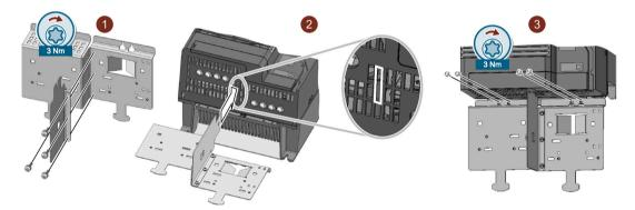
Use the shield plate provided for strain relief of the line and motor cable – as well as the shield support for the motor cable.
