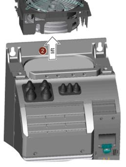
2. Install the new fan module in inverse sequence. By inserting the fan module, you establish the electrical connection between the converter and fan module.
