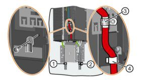
4.2 Connecting the line and motor cable at the converter
