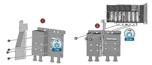
You have correctly mounted the EMC connecting bracket and the shield plate.
