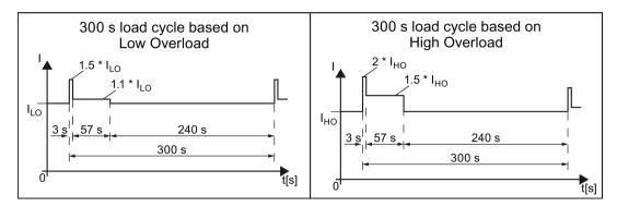
Figure 6-1 "Low Overload" and "High Overload" load cycles
