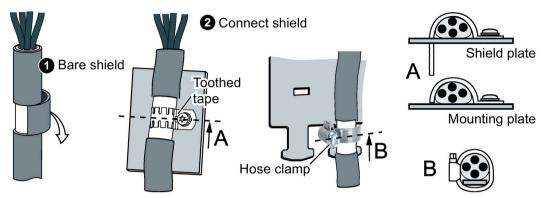
Figure 3-4 Examples for EMC-compliant shield support
