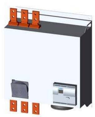
SIRIUS SOFT STARTER, VALUES AT 400V, 40DEGREES, STANDARD: 1214A, 710KW, INSIDE DELTA: 2103A, 1200KW, AC 200-460V, AC 230V, SCREW TERMINALS
